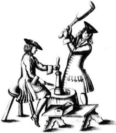
Figure 5. The manufacture of rockets in the Karlskrona pyrotechnical laboratory (drawing in the Karlskrona Naval Museum probably by Daniel Grundell), c. 1700-1716.
